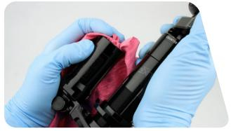
To check the bleed quality, install the IFP Height Tool into the IFP reservoir and apply force to the IFP Height Tool (approximately 25 lbs). The IFP should feel firm and should not compress. If the bleed check window is compressed beneath the edge of the reservoir, the system will need to be re-bled. To re-bleed the system, remove the IFP reservoir and the IFP, and return to step 4.
