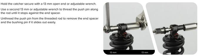
If the bushing pin did not remove easily, unthread the push pin from the threaded rod to remove the end spacer, then reinstall the push pin onto the threaded rod.
