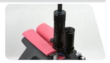
Remove the IFP reservoir valve cap. Depress the Schrader valve and release all air pressure from the IFP reservoir.
