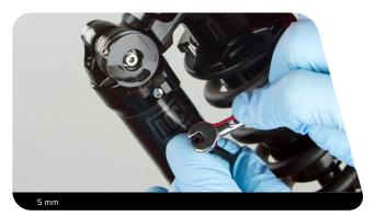
Install the threaded ferrule and housing into the cable hanger, then tighten the ferrule lock screw until it is flush with the cable hanger.
