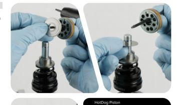
Separate the piston from the upper shim stack, still on the hex wrench or pick, and remove it. Slide the HotDog Piston onto the hex wrench or pick, with the "HotDog" side of the piston facing the end of the hex wrench.
