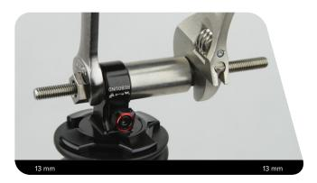
Unthread the catcher from the threaded rod. Remove the tool from the shaft eyelet and discard the bushing.
