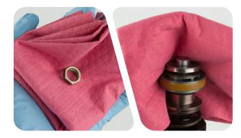
Slide the main piston assembly and top out plate off the shaft and onto a small hex wrench or pick.
