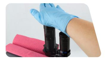
Install the IFP into the damper body with the flat side visible. Use a metric caliper or ruler to push the IFP into the reservoir to a depth of 20 mm.
