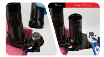
Pour suspension oil into the IFP reservoir until it is level with the top of the IFP reservoir. Oil will begin to bleed into the damper body.
