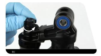
Turn the preload adjuster counter-clockwise until there is a large gap between it and the spring.
