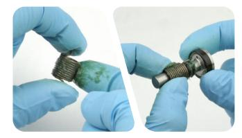
Install the cam and spring into the cam housing, and rotate the cam until the spring tang falls into the tang hole. The cam should be flush with the end of the cam housing.
