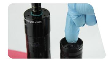
Remove the retaining ring from the IFP reservoir.
