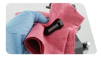
Remove the shock from the vise, and install grooved soft jaws into the vise. Gently clamp the cam into the groove in the soft jaws.
