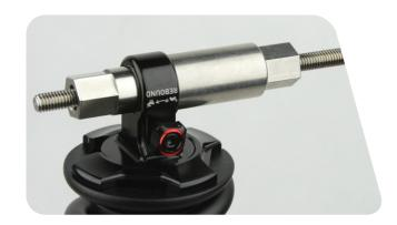
Hold the catcher secure with a 13 mm open end or adjustable wrench. Use a second 13 mm wrench to thread the push pin along the rod until the push pin pushes the eyelet bushing out of the eyelet.
