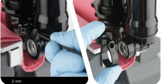
Loosen the IFP reservoir from the eyelet.
