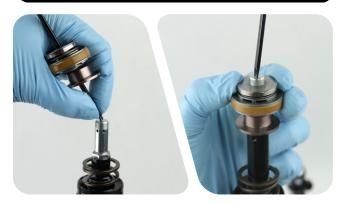
Thread the nut onto the damper shaft. Tighten the main piston nut. Remove the assembly from the vise.
