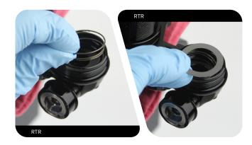
15 Install the compression assembly into the reservoir mount. Push the compression assembly into the reservoir until it stops.
